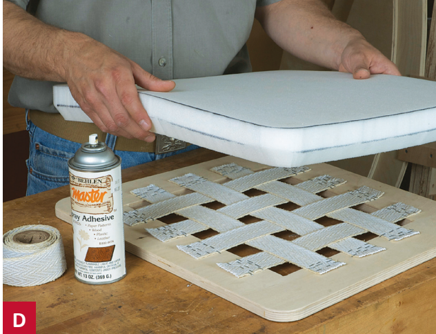
Align foam with plywood carefully. Spray on adhesive and apply downward pressure to ensure good bond.
