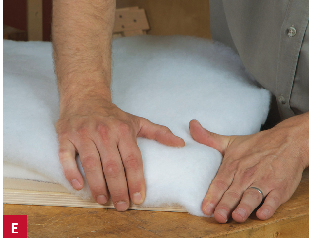
Fit the polyester fiber onto the foam. Trim back any extra that runs over the edge of the plywood.
